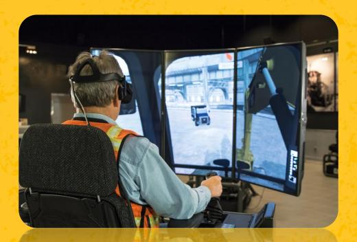
Real-time simulation software and hardware cabin integrated with the motion system, which also has an operator module, a special effects sound module, and is equipped with a monitoring system module for several types of heavy equipment.
